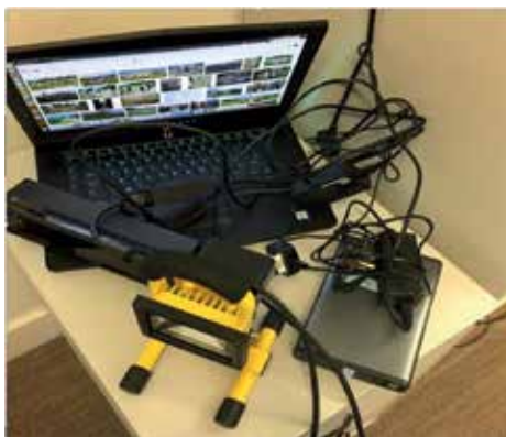
Kinect scanning kit: laptop, Kinect, battery, LED lamp.
