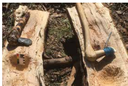
Results after 90 minutes: both mortises some 130 mm wide but that cut by the flint axe some 20 mm deeper and with near vertical sides
