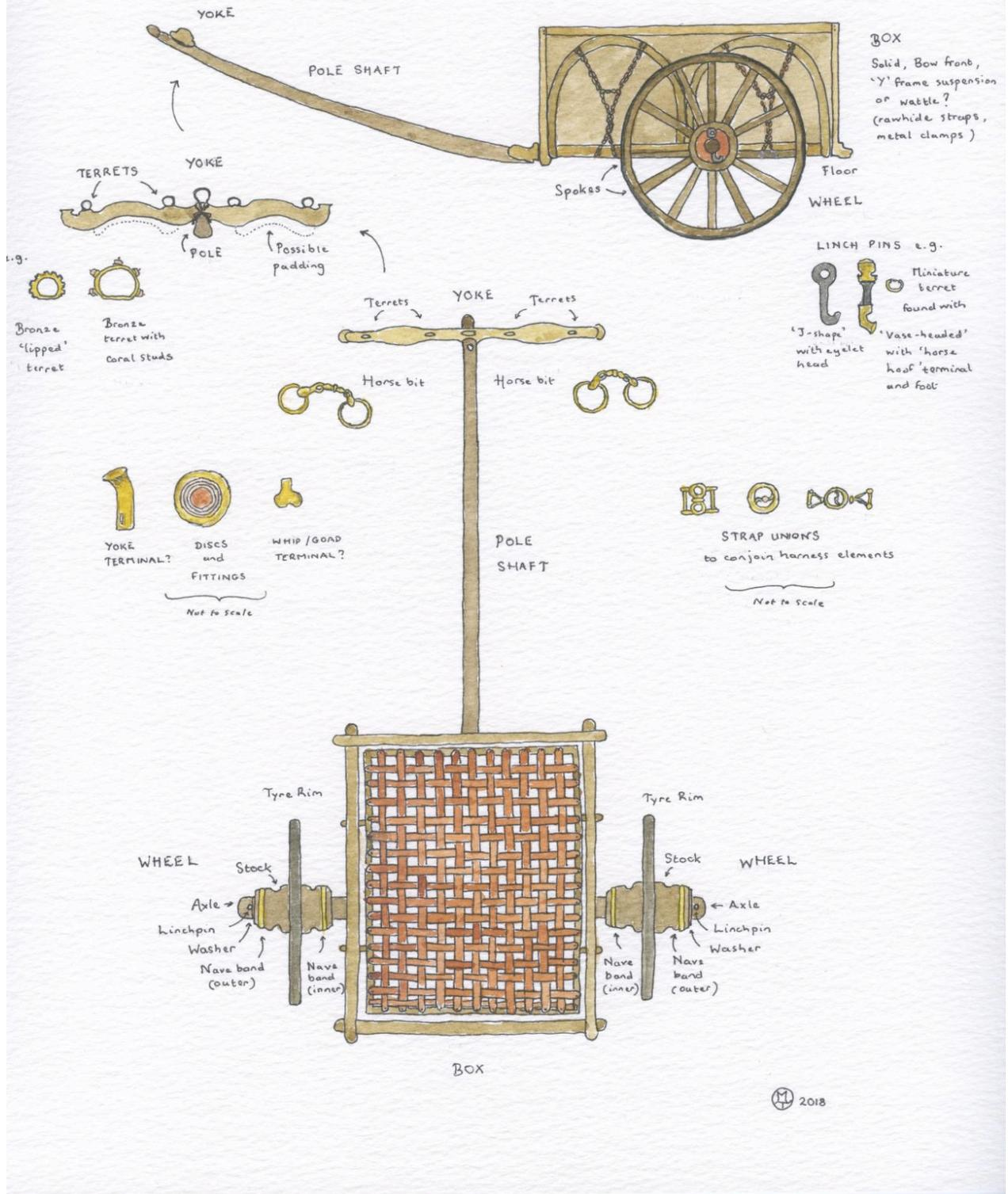
Figure 2. Reconstruction of an Iron Age chariot, showing key components.
